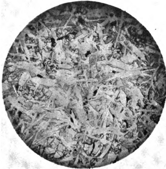
A. PHOTOMICROGRAPH OF DIABASE, DAVIDSON COUNTY, N. C.; 30 DIAMETERS; AUGITE, OLIVINE, PLAGIOCLASE AND MAGNETITE, OPHITIC TEXTURE. ORDINARY LIGHT.
